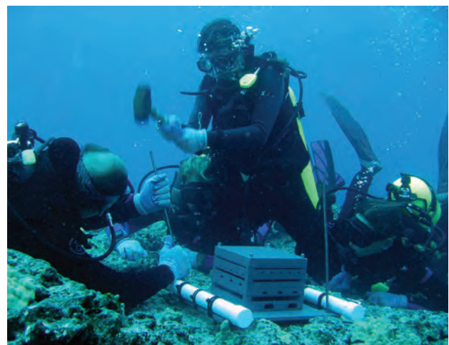
8. Artificial Reef Monitoring Structures are small boxes made out of PVC with many tiny holes for invertebrates such as crabs, and mollusks to inhabit. They are designed to mimic the reef environment, and after a year or two the boxes are removed from the reef and studied to see what organisms settled inside and on top of them. Source: Andy Collins, National Oceanic and Atmospheric Administration
